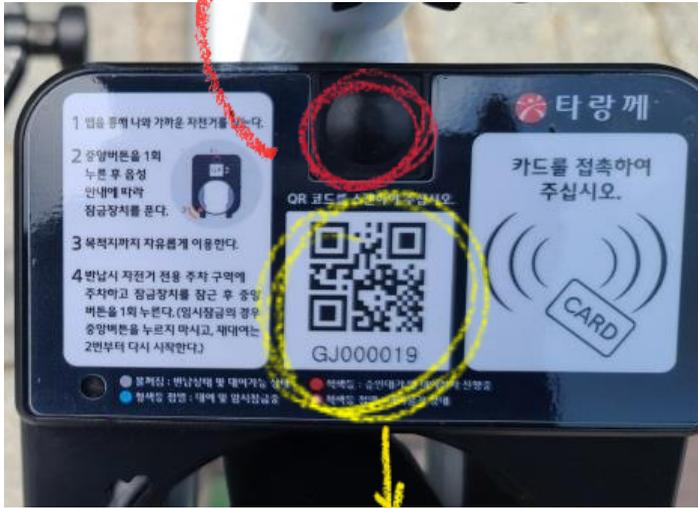
3. Scan QR-Code then the mechanism would be unlocked. Then use it.
